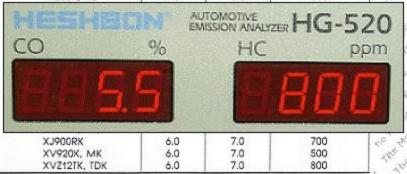
Yamaha to their credit took the high road by providing its dealers carbon monoxide (CO) specifications for all its models, to be set using an exhaust gas analyzer (EGA). This is a superior method for setting idle mixtures. However, to my knowledge, no other Japanese powersports manufacturer ever supported EGA use.
