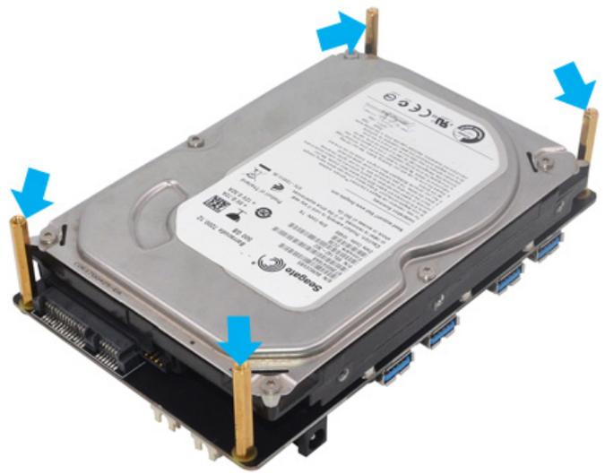
**11** Push the second X835 up through the M/F M3\*40 spacers on the underside of the first X835 and screw down (Spacer F/F M3\*32mm, if add one more X835 then using a spacer M/F M3 x40mm) until it is hand tight.
